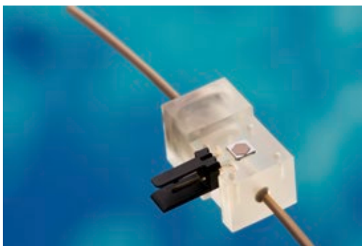
Smallest micropump in the world with dimensions of 3,5 \times 3,5 \times 0,6 \text{ mm}^3 © Fraunhofer EMFT / Bernd Müller
