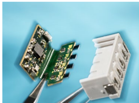
The contactless electronic sensor system serves as an intelligent diagnostic interface for the Internet of Things (IoT), enabling reliable condition monitoring of the environment using the example of a printed circuit board connector (Smart Mechanical Electrical Connector, SmeC)
