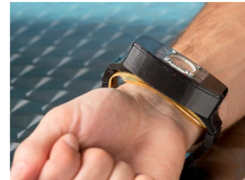
Mobile blood pressure measurement using micropumps
