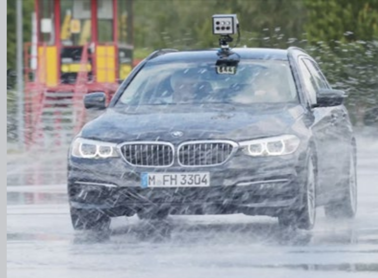
Original prototype of the early warning system for detecting aquaplaning and black ice undergoing testing
