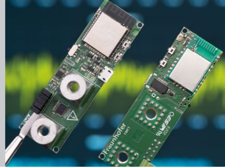
Miniaturized reverb-based current sensor module
