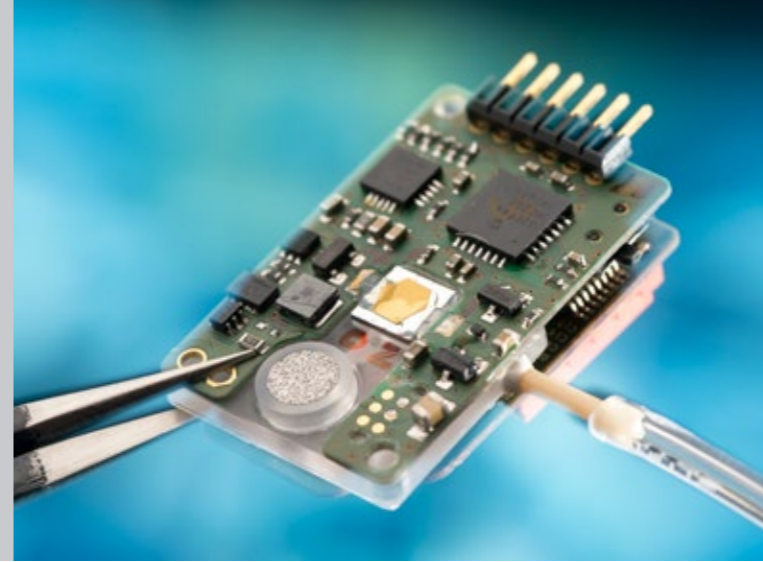
Prototype of a fine dust particle sensor based on the capacitive measurement principle for the measurement of PM10, PM2.5 and PM1.0 particles. It consists of a fluidic module including filter, micropump and fluidic channel for aerosol supply, and the sensor module for particle detection.
