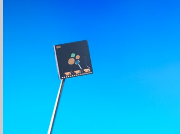
CMOS ion-sensitive field-effect transistor with controllable floating gate (FG-ISFET)
